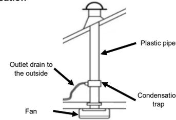
To avoid the backflow of condensation into the fan in ceiling installations it is good practice to fit a condensation trap to the vertical outlet duct of the fan. With **thru-the-wall installation** fit the duct in an approx. 5° angle down to outside.
