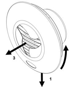
To remove front cover assembly, first make sure the fan is off, isolated from the power supply and the iris shutter is fully closed.
