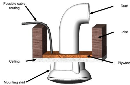
When surface mounting the iCON 30 and iCON 60, the mounting skirt provided should be used. The mounting skirt should be fixed, with the screws provided, into the support. The fan is then fitted into the skirt.
