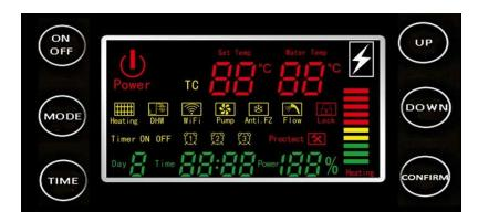
Press ON/OFF button to turn boiler on – Standby
