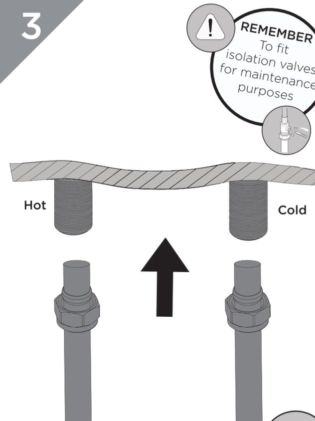
Connect the hot and cold water supplies to the threaded tails.
