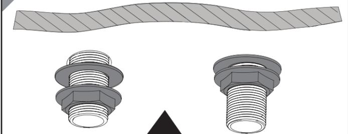
Secure the taps to the bath by using the washer and metal backnut below the basin.
