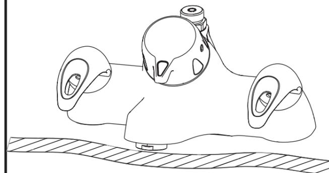
Connect the hot and cold water supplies to the threaded tails.
