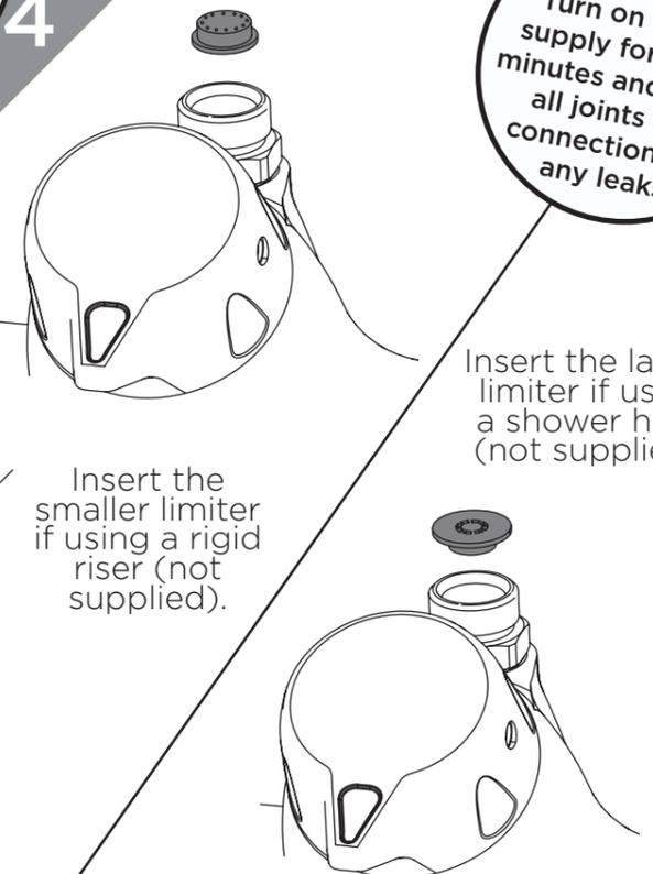
Insert the smaller limiter if using a rigid riser (not supplied).
