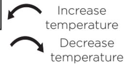
Turn the knob anti-clockwise to the maximum flow/temperature position.
