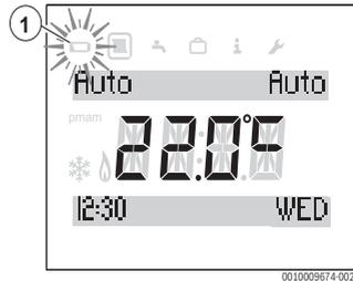
Fig. 16 Low batteries display
