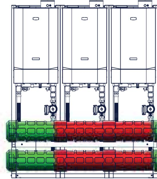
STANDARD HEIGHT INSULATION STARTER KIT + STANDARD HEIGHT INSULATION CONTINUATION KIT + STANDARD HEIGHT INSULATION CONTINUATION KIT
