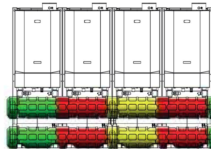
LOW HEIGHT INSULATION STARTER KIT + LOW HEIGHT INSULATION CONTINUATION KIT + LOW HEIGHT INSULATION JOINED HEADER KIT + LOW HEIGHT INSULATION CONTINUATION KIT
