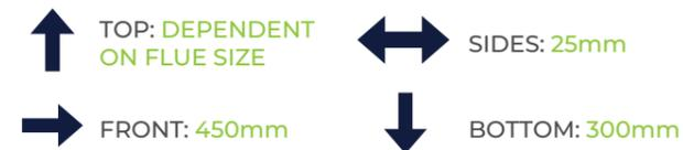
CLEARANCE BETWEEN MULTIPLE BOILER INSTALLATIONS: 25mm
