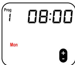
**Step 2:** Press and hold STANDBY for 5 seconds to enter the copy day setting.
