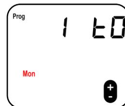
**Step 5:** Press the STANDBY button to copy the programs. The 'TO' will flash to confirm the programs have been copied.
