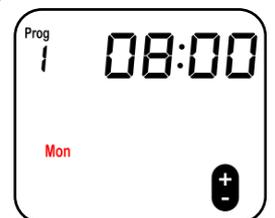
**Step 6:** Press the MENU button. Prog 1 in the top left of the display should flash. Use the + button to increment this to Prog 2. (Note: you can cycle between the different programs using the + and - buttons)
