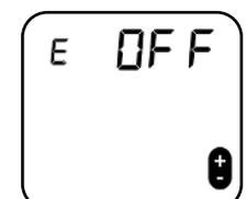
If this is **ON** the back light will be permanently on when the heater is active.
