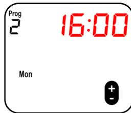
**Step 8:** Press the MENU button. The temperature should flash. Use the + and - buttons to select a frost protection temperature.
