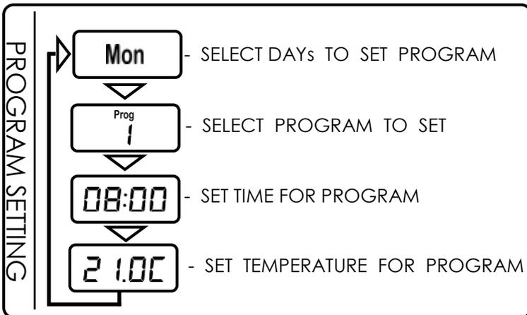
The timer is set to 5 days and 2 days as default. This section provides an example of how to set the program for Monday to Friday. The example will program the timer to maintain 21°C from 08:00 until 16:00. It will maintain 4°C from 16:00 onwards. It does this by setting the programs as follows;
