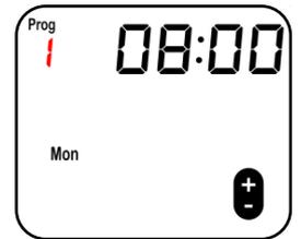
**Step 3:** Press the MENU button. The time should flash. Use the + and - buttons to set the time you want the heating to switch on.
