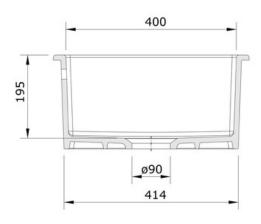
NB: Due to manufacturing processes this sink may have a +/- 3mm tolerance on the measurements.
