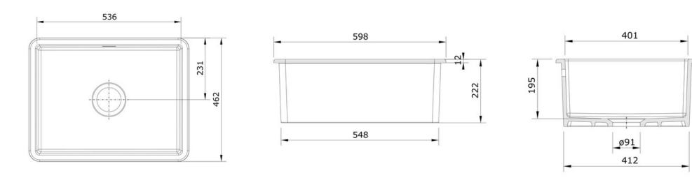
NB: Due to manufacturing processes this sink may have a +/- 3mm tolerance on the measurements.
