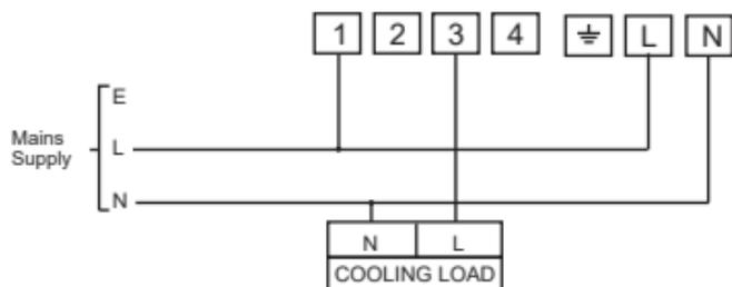
C-Stat wired to control a cooling load. When necessary the C-Stat should be used in conjunction with a contactor.
