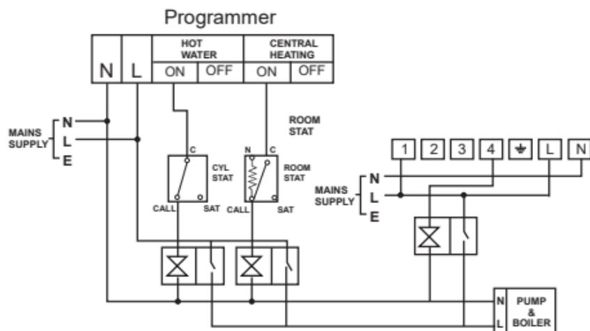
C-Stat controlling a secondary heating zone on a fully pumped system with existing programmer and two spring return valves with auxiliary switches.
