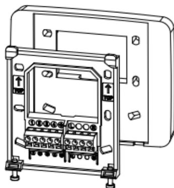
The mains supply terminals are intended to be connected to the supply by means of fixed wiring.
