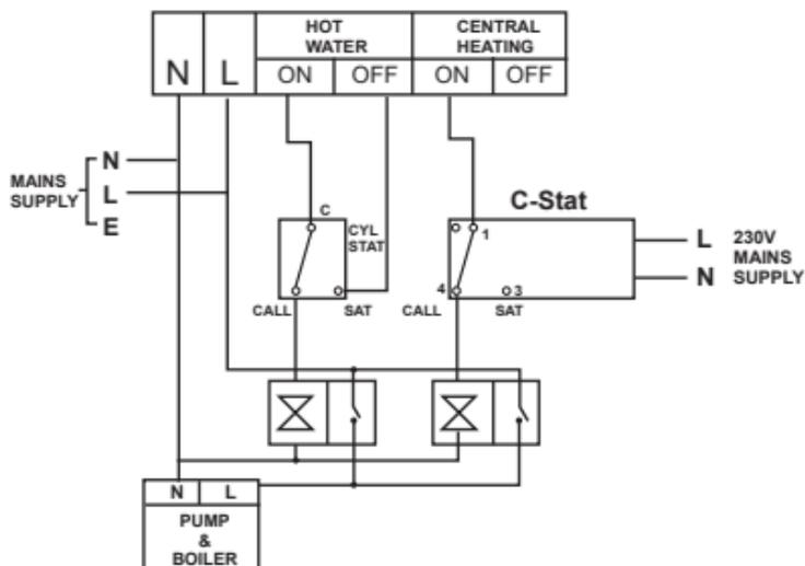
C-Stat replacing a conventional room thermostat on a fully pumped system with an existing programmer and two spring return valves with auxiliary switches
