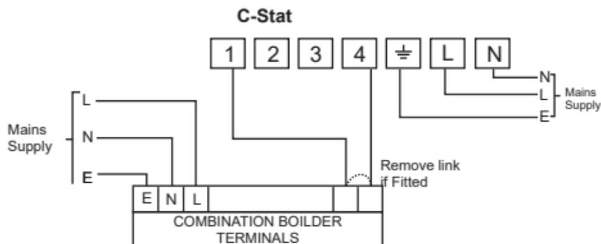
C-Stat controlling typical combination boiler installation. For precise termination connection information please refer to the boiler manufactures instructions
