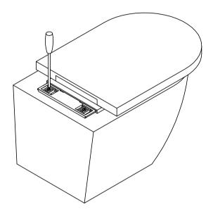
WITH THE FIXING PLATE AND BOLT SETS IS IN POSITION, SLIDE THE PLATE BACK INTO THE HINGE PLATE 5mm ONLY AS THIS WILL ALLOW ACCESS FOR TIGHTENING THE BOLTS.
