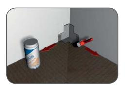
Step 10 Place the waterproofing internal corners into the internal corners of the shower tray and push firmly into the Pro-SEAL tape sealer. Apply a further thin layer of Pro-SEAL tape sealer over the edges of the waterproofing internal corners.
