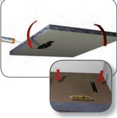
Step 6 Spread Fix-KST adhesive across the surface of the Substrate Element using a notched adhesive trowel to leave just the right amount of adhesive on the shower base.
