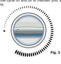
NOTE: If the heater does not come on when the thermostat is set to a low number, this is normally because the room is warmer than the thermostat setting and is not a fault.
