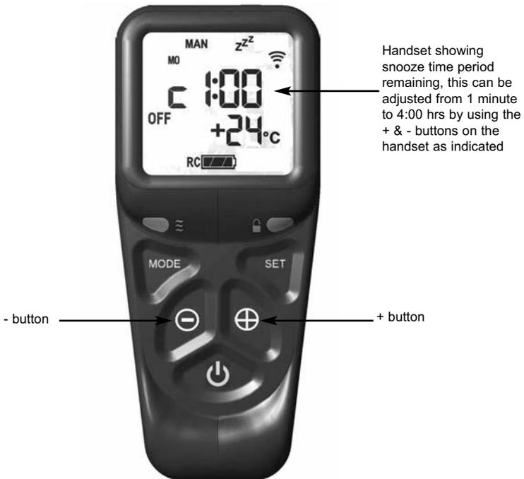
5.6.1.8 To adjust the snooze period use the + and - buttons to increase or decrease the snooze period for any period between 1 minute and 4:00 hours.
