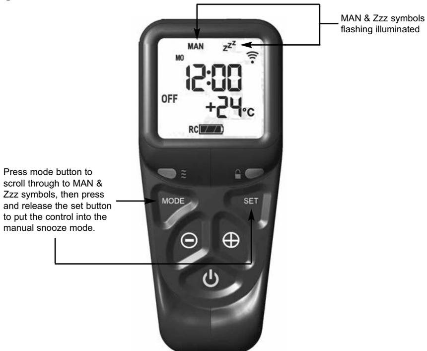
5.6.1.6 Pressing the set button again will now show you the snooze time period remaining. The snooze time period can be adjusted by pressing the + or - buttons on the handset. This time period can be set ranging from 1 minute to 4:00 hours.
