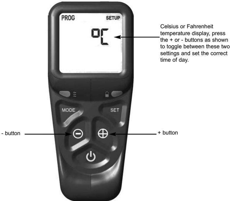
3.5.7 As shown above in figure 18 the time on the handset can now be set by using the + and - buttons to change the hour to the correct hour then press SET to store and to move to setting the minute. Repeat this process for setting the minute to the correct minute then press SET to store.
