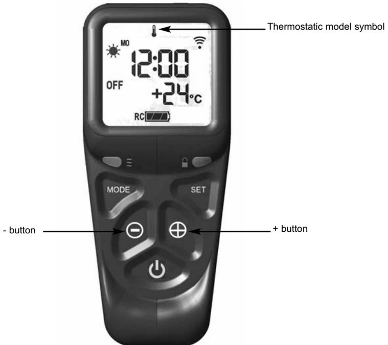
5.6.2.3 Press the set button again to see the temperature setting that is set (the default is 24 degrees celsius). If a different set temperature is required, whilst the display is showing this set temperature, press the + and - buttons to alter this setting, press the set button to store the required temperature, or alternatively the handset can be left for a few seconds and the temperature will be stored automatically.
