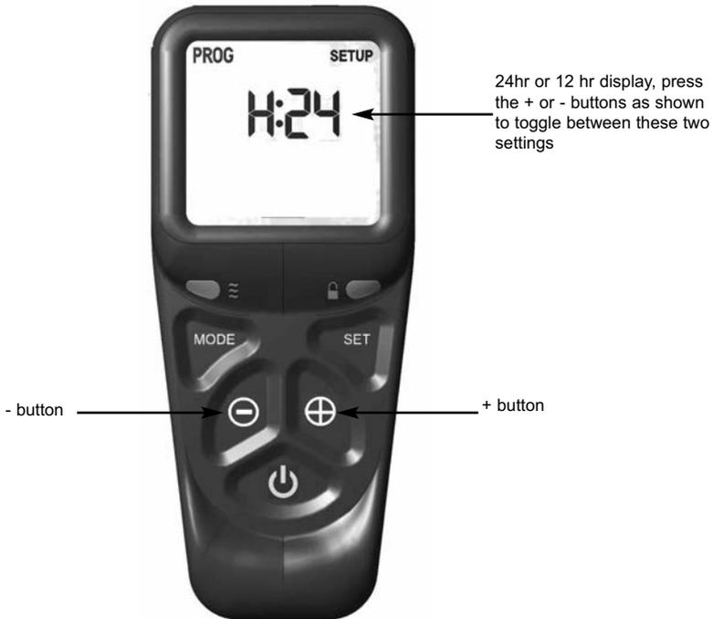
3.5.4 When the 24hr or 12hr time display option has been chosen and you are ready to confirm the setting you want press the SET button on the handset to progress to setting the day of the week as shown overpage in figure 19.
