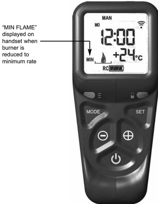
3.6.4 To increase the heat input level of the fire's burner hold the handset as described in section 3.5.1 to unlock the keypad then press and release the + button. Pressing and releasing the + button will increase the heat input level one step at a time. Pressing the + button continuously will move the heat input level to the maximum.
