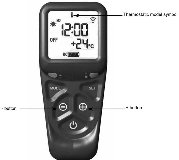
3.7.2.3 Press the set button again to see the temperature setting that is set (the default is 24 degrees celsius). If a different set temperature is required, whilst the display is showing this set temperature, press the + and - buttons to alter this setting, press the set button to store the required temperature, or alternatively the handset can be left for a few seconds and the temperature will be stored automatically.
