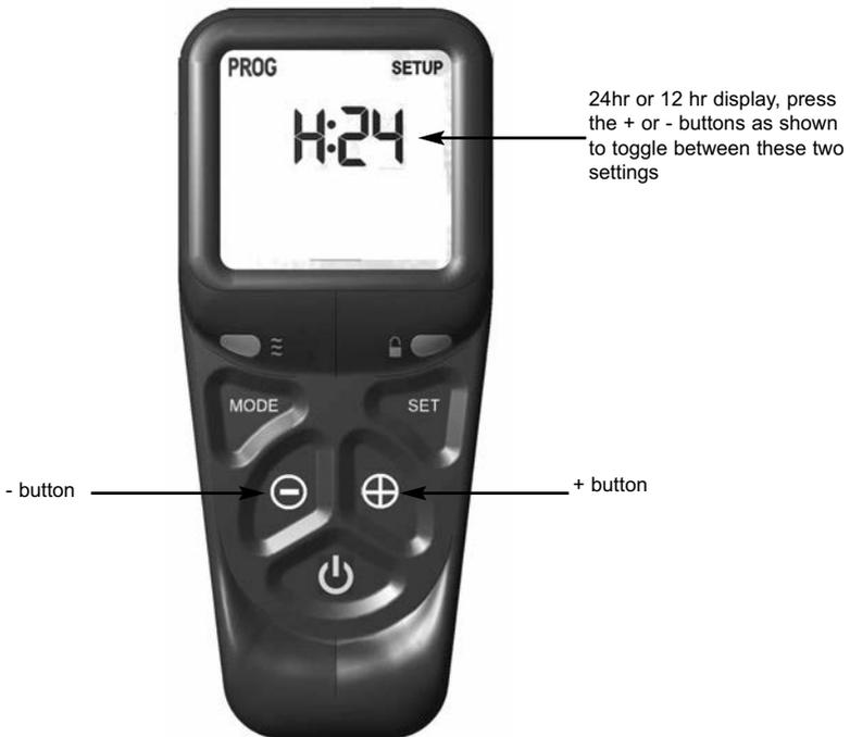
5.5.4 When the 24hr or 12hr time display option has been chosen and you are ready to confirm the setting you want press the SET button on the handset to progress to setting the day of the week as shown overpage in figure 9.
