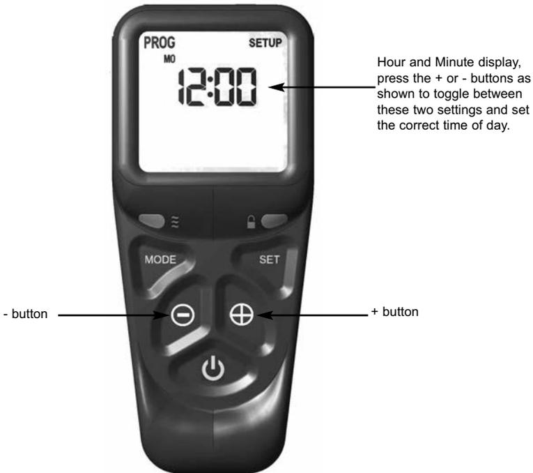
5.5.7 As shown above in figure 9 the time on the handset can now be set by using the + and - buttons to change the hour to the correct hour then press SET to store and to move to setting the minute. Repeat this process for setting the minute to the correct minute then press SET to store.
