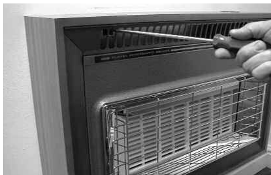
Fig. 10 Removing the Upper Outer Case Fixing Screws
