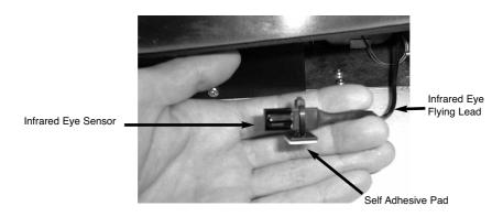
Remove the backing paper from the self adhesive pad and position the infrared eye in the corner of the ashpan cover, so that the infrared eye is flush with the front edge of the front bezel cover, as shown below in Fig. 8. Check the operation of the handset, as detailed in Section 3.3 and adjust the position of the infrared eye if necessary.
