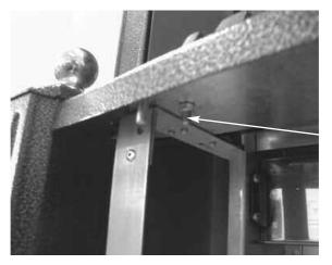
Front bezel retaining screws (1 off each side)
