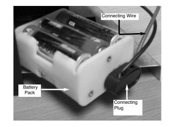
d) Replace the battery pack into its mounting cradle below the fire / burner and re-assemble in reverse order.
