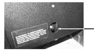
Emergency Shut Off Switch Position on Control Panel.
