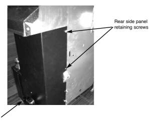
Front retaining screw on the underside of the leg support bracket
