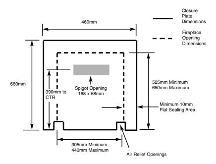
Apply a smoke match to the flue spigot opening in the closure plate and observe the smoke. If there is a definite flow into the opening then proceed with the installation. If there is not a definite flow into the opening, pre-heat the chimney for about two minutes and retest for flow. If there still is no definite flow into the opening, the chimney may require attention. DO NOT FIT THE FIRE-SEEK EXPERT ADVICE.
