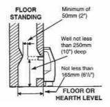
1.8.2 Fitting to Pre-Fabricated twin wall metal Flue Boxes.
