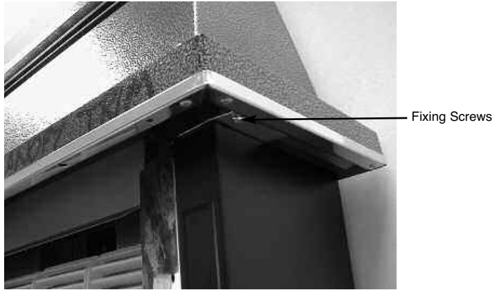
Fig. 7 Removing the Upper Outer Case Fixing Screws
