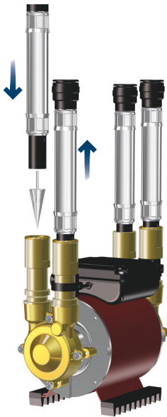
Fig. 17 Fitting the strainer basket
