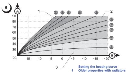
A Heating flow temperature B External temperature
