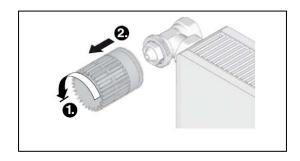
4. Put the Valve baseplate on the valve use adaptor if necessary
