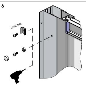
WHEN THE FRAME IS READY TO BE FIXED, DRILL THROUGH THE HOLES IN THE WALL PROFILE WITH A 3mm DRILL. (MAKE SURE YOU ONLY DRILL THROUGH ONE WALL THICKNESS) THEN FIX THE FRAME WITH ITEMS 26, 28\* & 29\* \* IF YOU HAVE THE OPTIONAL SCREW COVER PROFILE (ITEM 7) DO NOT USE ITEMS 28 & 29, FIT ITEM 13 UNDER THE SCREW.
