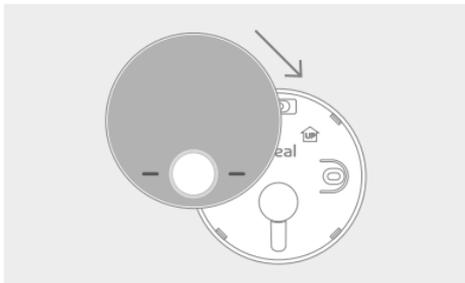
4. Locate the front housing (display) in position parallel to the rear housing and clip into place.
