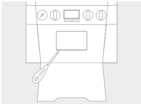
5. Locate the blanking plate on the front of the boiler and remove carefully with a small flat bladed screwdriver.
