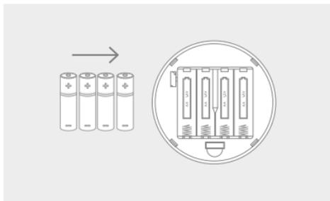
2. Insert the 4 AA batteries provided into the front housing of the Halo. Pay close attention that the orientation of the batteries is as indicated in the housing.
