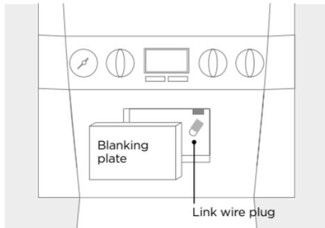
6. Remove link wire plug and keep in a safe place.
