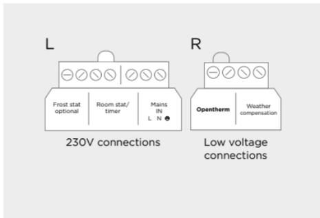
2. Locate the wiring terminals (230V connections are on the left and low voltage on the right).
