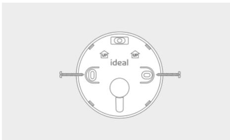
2. If no trim plate is required, use the rear housing of the Halo to position the unit on the wall, alternatively secure rear housing to trim plate. Take care not to overtighten the screws.
