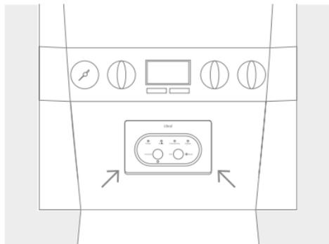
8. Push fit the Halo Smart Interface into the boiler aperture.
