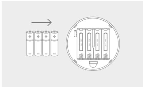
3. Insert the 4 AA batteries provided into the front housing of the Halo. Pay close attention that the orientation of the batteries is as indicated in the housing.
