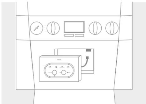
7. Connect the plug on the Halo Smart Interface to the connector in the aperture.
