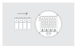
2. Insert the 4 AA batteries provided into the front housing of the Halo. Pay close attention that the orientation of the batteries is as indicated in the housing.
