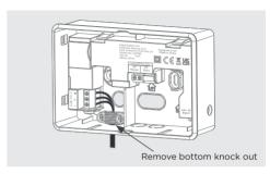
4b. Surface cable mounting; From the fuse spur wire the Live, Neutral and Earth into the left hand side connections in the Smart Interface Bracket marked L, N, (E). Using the cable clamp provided.
