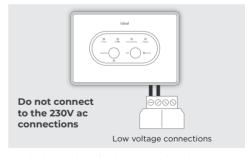
10. Take the cable that is wired into the bracket OpenTherm Master terminals and connect into the OpenTherm connections in the boiler ensuring it is run through the strain relief (in new boilers remove the link positioned here before wiring).
