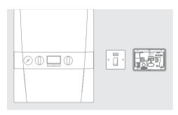
Locate the Smart interface bracket in a suitable location close to the boiler and fuse spur as the bracket is hard wired to both.
