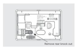
4a. Rear cable mounting; From the fuse spur wire the Live, Neutral and Earth connections into the left hand side connections in the Smart Interface Bracket marked L, N, (E).
