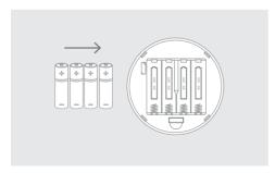
3. Insert the 4 AA batteries provided into the front housing of the Halo. Pay close attention that the orientation of the batteries is as indicated in the housing.
