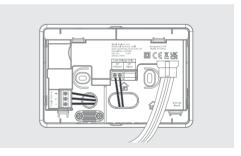
6. Install the Smart Interface by connecting the plug on the Smart Interface to the connector in the bracket.
