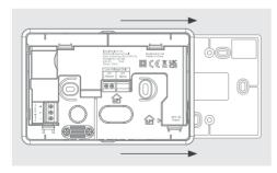
2b. To mount over the electrical box, place the bracket over the electrical box and fix into place.
