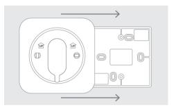
The Halo can be installed with or without the provided trim plate.
