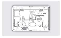
2a. To mount directly onto the wall, mark and drill 2 mounting holes and fix the bracket to the wall using suitable fixings for the wall type.
