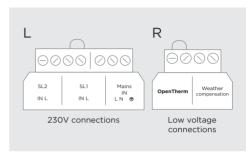
Locate the wiring terminal within the boiler control box (230V connections are on the left and low voltage on the right).
