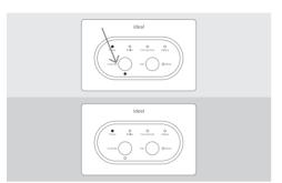
Check the Smart Interface connection to the boiler by pressing the override button. The override LED should be green and the boiler will fire. Press the override button again to switch off the boiler, the override LED should now go out\*
