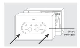
7. Carefully push the Smart Interface into the bracket.
