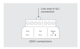
If an existing 230V signal is already installed remove any existing wiring from the 230V connections and add the link wire into the SLI connections
