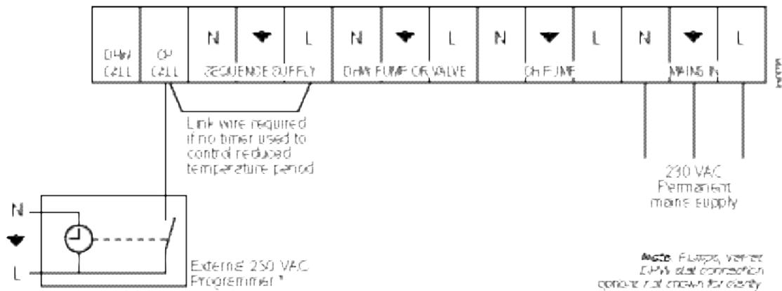
\* The switched live from external controls must be from the same phase supply as the boiler mains supply to ensure that when the boiler supply is switched off the controls are also isolated
