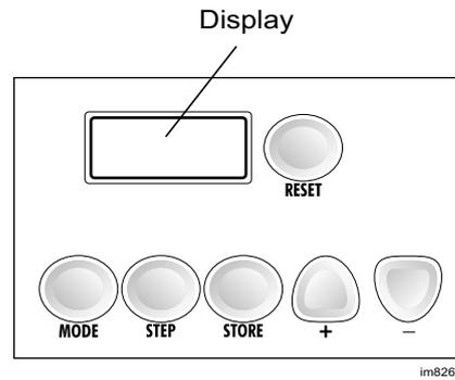
Code Mode is entered from standby mode by pressing and holding the 'mode' and 'step' buttons.
