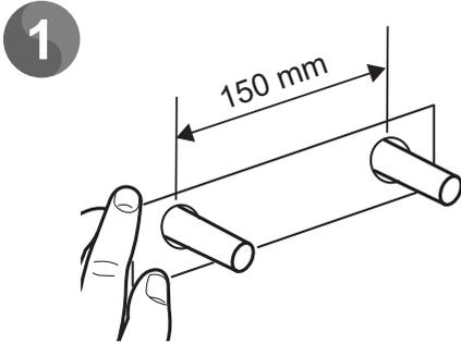
Fit the plastic pipe guide over the inlet pipes. Level the pipe guide and secure to the wall to hold in position. **Leave the guide in place and finish the wall.**
