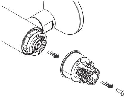
6. Temperature adjuster can be moved 3 positions in either direction, one position equals 1°C. Rotate adjuster anti-clockwise to increase temperature and rotate clockwise to decrease temperature.
