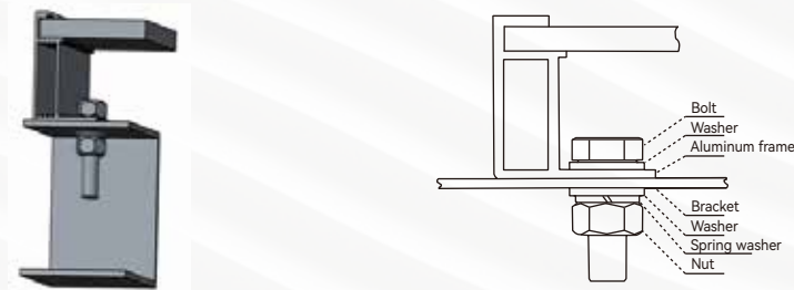
Figure 5 Bolt Installation of Mono-facial Modules
