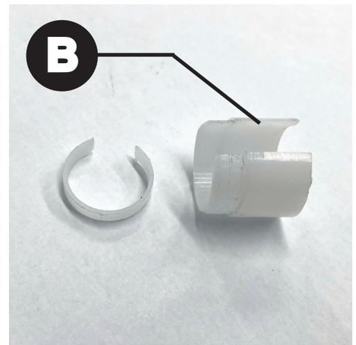
3. Take the anti legionella valve and identify the end with the female thread that screws onto the expansion vessel. Located here is a flat white plastic paddle (C) that will require cutting down by 3mm. The paddle already has a small crease at the desired break point and may break off without the need for a knife (D).
