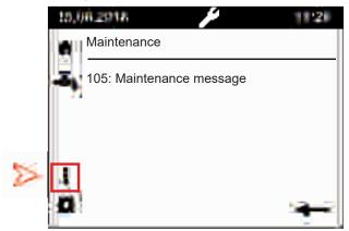
In this example '105: Maintenance message' is used to notify the user, the heater has been in operation for more than 12 months and requires a service inspection. When servicing has been completed, the service counter should be reset using parameter 7045, in the Service / special operation menu (see installation and maintenance manual section 9.2.1).
