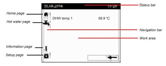
The water heater is operated by rotating 1 to move the selector over the screen then pushing 1 to select the item. When selected the item will be displayed as inverse and can then be changed by rotating 1 and the change is confirmed by pushing 1 (enter).
