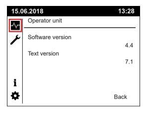
Details are shown for the software and text versions being used by the GUI, this may be useful to establish the level of updates applied to the heater.
