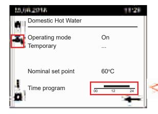
With the DHW page selected, rotate ① to highlight the time program field, then press enter to open the time clock setting page.
