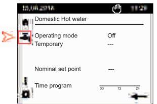
Outside of the programmed operation times for water heating, the operation of the water heater can be turned on for a single occasion where Hot Water will be heated to the nominal set point. The heater control returns to normal operation using pre-settings as soon as the hot water reaches set point.
