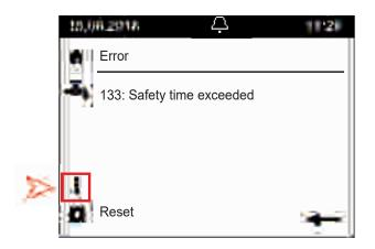
If the heater controls are unable to operate the gas burner or it detects a undesirable condition, the controls will put the heater into a "lockout" mode and the heater may be prevented from operating again, until manually reset.
