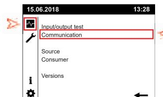
Highlight "Communication" by rotating ① and select the function by pressing enter.
