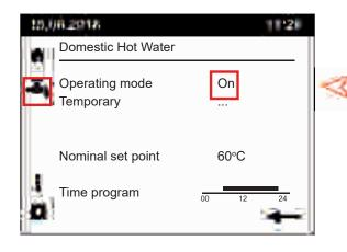
Rotate ① to select the operating mode, then press enter to select and change the mode to "On".
