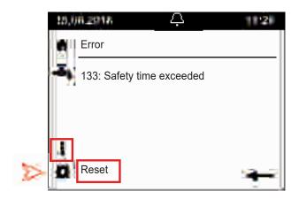
In this example the heater has gone into a lockout mode, because the gas supply has been interrupted. The resolution would be to re-establish the gas supply to the heater and then reset the error to restart heater operation again (see below).
