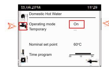
Select the Domestic Hot Water (DHW) page by rotating and pressing ① . Toggle to the operating mode and ensure that Domestic Hot Water is turned "On".
