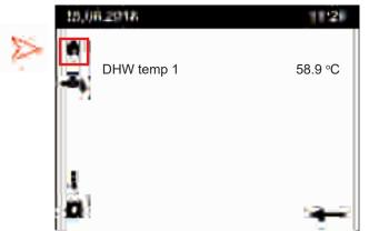
The home page for the heater GUI unit displays the most important information on the water heater and system operation mode. There are no settings that can be applied whilst in this screen.
