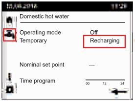
Change the "Temporary" field from "---" to "Recharging" and press enter to activate Temporary operation mode.
