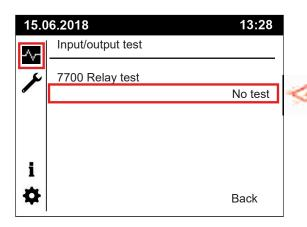
Once the testing has been completed, use 1 to change field "7700 Relay test" back to "No test" and the heater will revert back to normal control of the outputs.
