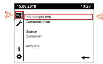
Highlight "Input/output test" by rotating ① and select the function by pressing enter.
