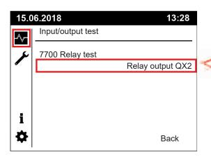
Rotate 1 to field "7700 Relay test" and press enter. Rotate 1 to select output to test. Press the enter to activate the desired output relay (see example above).
