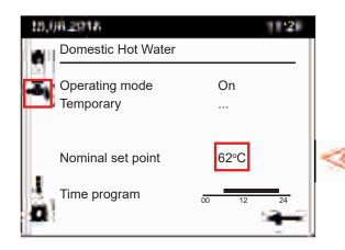
Using ① to highlight the "Nominal set point" press enter and enter a new value and then enter within 3 seconds to confirm.
