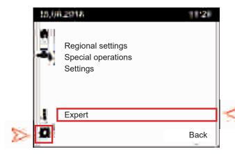
Using the Graphical User Interface, rotate 1 to select "Setup" page on the navigation bar and press enter to select. In the work area , rotate 1 to select "Expert" field and press enter to select.
