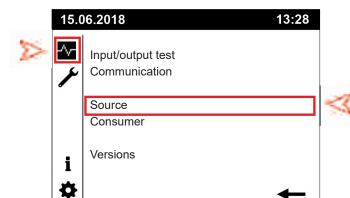
Highlight "Source" by rotating  $\ensuremath{\textcircled{1}}$  and select the function by pressing enter.
