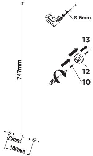
4. The telescopic section of the riser can adjust the height between 840-1170mm, loosen the fixing nut on the rail bracket, adjust to the desired height and re-tighten the fixing nut.
