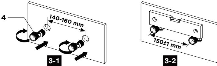
4. From the front, align the Eccentric Unions (4) with the Bar Valve (1) inlets. Screw Flange (3) to the ¾ inch section of the Eccentric Unions (4) protruding through the wall. Sealant can be used between the Flange (3) and the wall.
