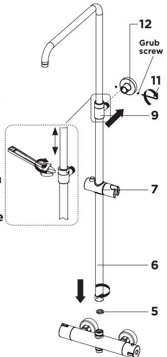
7. Tighten the fixing nuts of the shower tube using a suitable tool, taking care not to overtighten.
