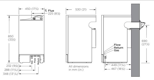
Flue pluming is a by-product of efficiency. Please be aware of terminal positions to avoid complaints. For full technical details please refer to the Installation and Servicing Instructions provided with the product. The flue duct must be inclined at a minimum of 1.5 degrees to the horizontal to allow the condensate to be properly drained if using flue extensions.
