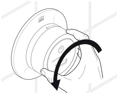
Adjust the temperature indicator in accordance to the table below to set the desired maximum temperature.
