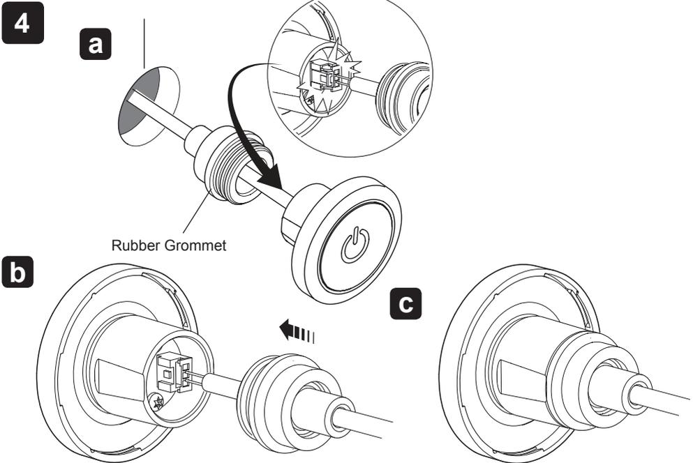
Connect the cable to the back of the ON/OFF button.
