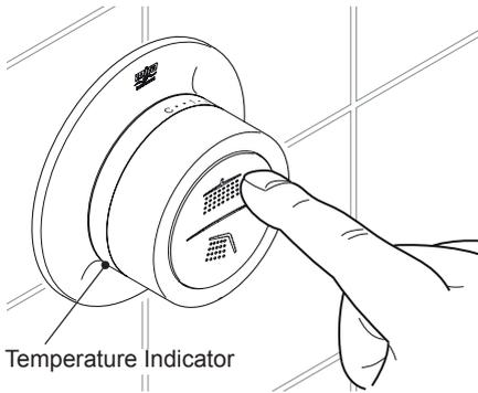
Hold down the Overhead Shower Button (top half) for 10 Seconds approx. until the Temperature Indicator light pulses on/off.
