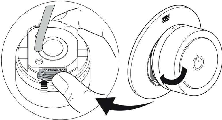
Locate the top of the interface in the backplate and press down on the bottom button as you install in position.
