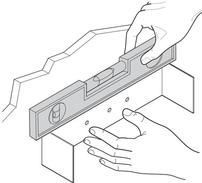
Position the installation template (supplied) at the position on the wall where you intend to install the interface. Make sure that the template is level.
