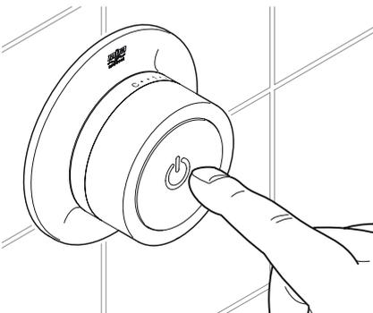
Hold down the On/Off Button for 10 Seconds approx. until the Temperature Indicator light pulses on/off.
