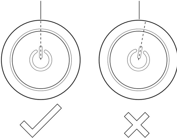
Carefully, visually align the symbol to the vertical line on the wall
