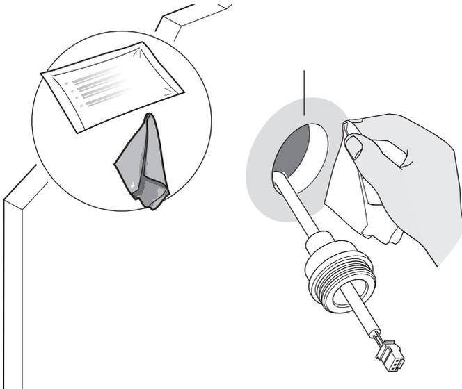
Using the cleaning wipe (supplied) clean the surface around the mounting hole.
