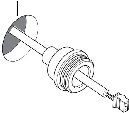
Route the cable from the digital valve through the hole in the wall.
