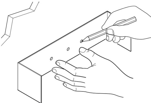
Mark the positions of the fixing holes on the wall.
