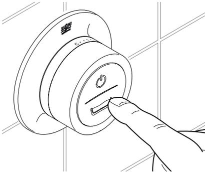
**Bath Fill Preset** – Push down the plug in the bath. Hold down the Bath Symbol Button (bottom half) for 5 Seconds approx. until the Bath Symbol Button flashes. Press the Bath Symbol Button (bottom half) to start the Bath filling. Rotate the Chrome Bezel to adjust the temperature indicator to set the temperature. On reaching the ideal fill level and desired temperature, press the Bath Symbol Button (bottom half) to stop the water & save the Bath Fill Preset.
