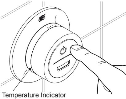
Hold down the On/Off Button (top half) for 10 Seconds approx. until the Temperature Indicator light pulses on/off.
