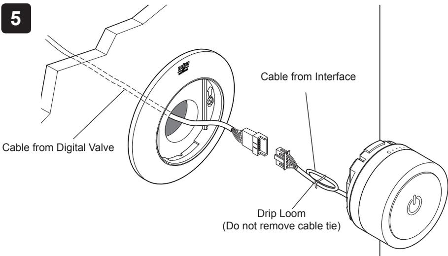
Connect the cable on the back of the interface to the cable that comes from the valve.
