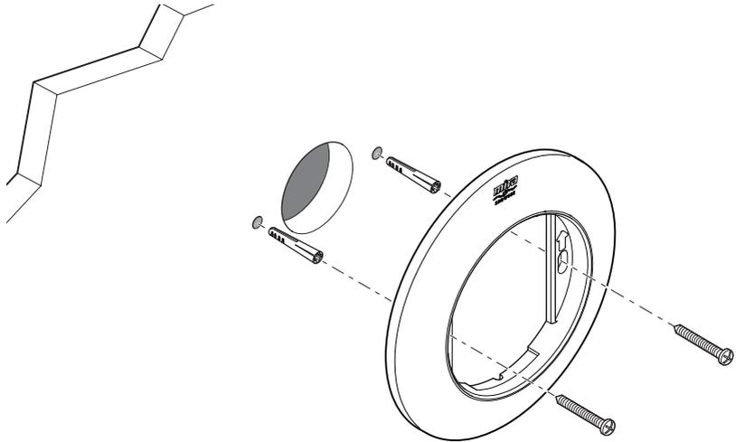
Fit the backplate to the wall in the orientation shown using the fixing screws (supplied). Tighten by hand, do not over tighten.
