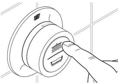
Hold down the Overhead Shower Button (top half) for 10 Seconds approx. until the Temperature Indicator light pulses on/off.
