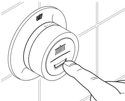
Bath Fill Preset temperature will calculate the average temperature over the Preset fill duration & take into account adjustments made to the User Interface rotary temperature dial during this time period.
