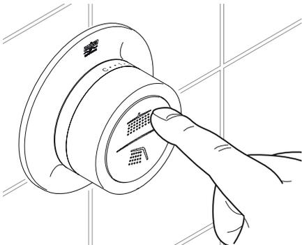
Press the Overhead Shower Button to set the maximum temperature. The temperature indicator light will flash twice to confirm the setting has been completed.
