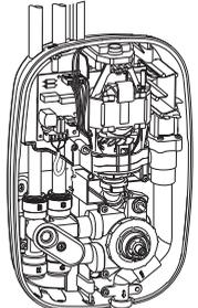
Fit the full blanking plate to the bottom of the case.
