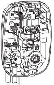
14. Locate the shower unit on the inlet supplies and push the inlet manifold onto the pipework until resistance is felt.
