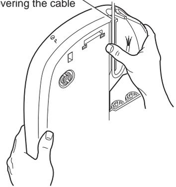
5. Loosen the three cover securing screws and remove the shower unit cover.
