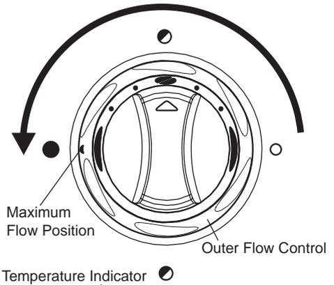
5. Rotate the inner temperature control anticlockwise to check the hot supply and clockwise to check the cold supply.
