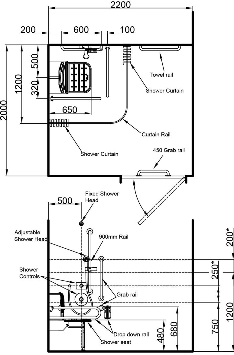
Above is for guidance only, refer to relevant building regulations (See data sheet for pack components).
