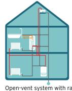
Open-vent system with raised tank to improve flow rate
