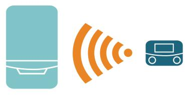
"Would you like weather compensation control to make your system more efficient?" Weather compensation control is an optional control available for modern boilers. It works by monitoring the temperature outside and using this information to help the boiler work as efficiently as possible.
