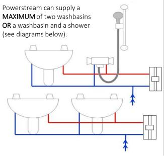
If connected to a mixer tap, it should be a **NON-**Thermostatic mixer tap; water mixes at the outlet pipe only.
