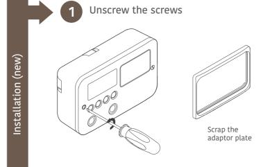
Note: The supplied Adaptor plate is ONLY required when retrofitting the E7\* onto an existing Electronic 7 or Economy 7 quartz back box.
