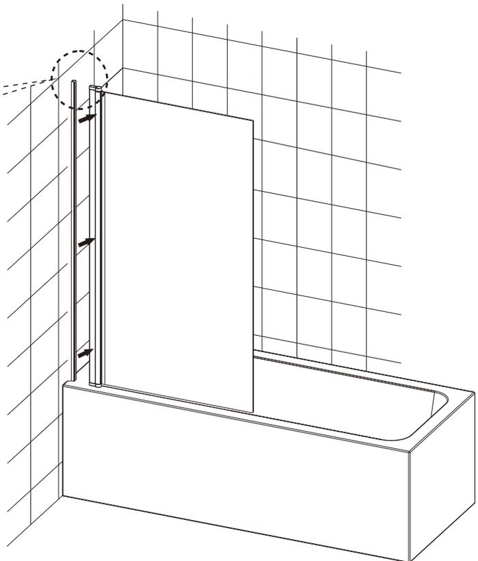
**NOTE:** To ensure the screen is parallel to the bath hold the top of the hinge and move the whole screen back or forwards to adjust before carrying out step 3.
