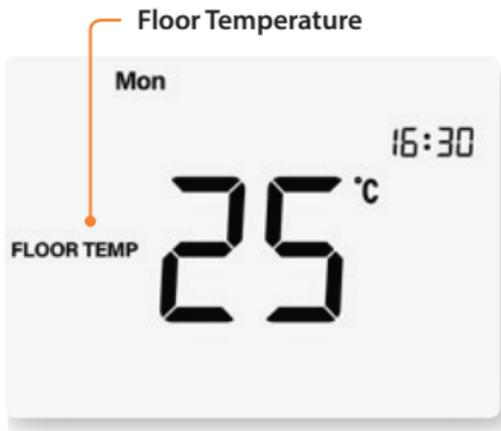
When the thermostat is set to use both sensors, the room temperature will be displayed. To view the floor temperature, press and hold the **A** key until the Floor Temp is displayed on screen.
