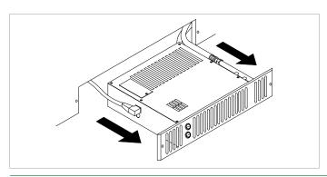
**4.** Disconnect the power plug from the side of the unit.
