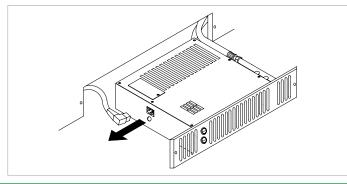
5. Connect the receiver unit between the power cable and the heater.
