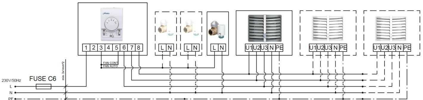
**3. Connecting HEATER units with INTELLIGENT panel.**
