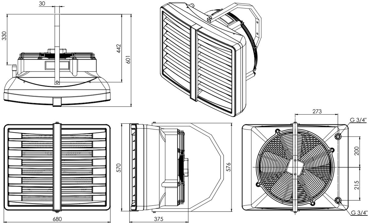
**DIMENSION AND BASIC TECHNICAL PARAMETERS HEATER ONE**
