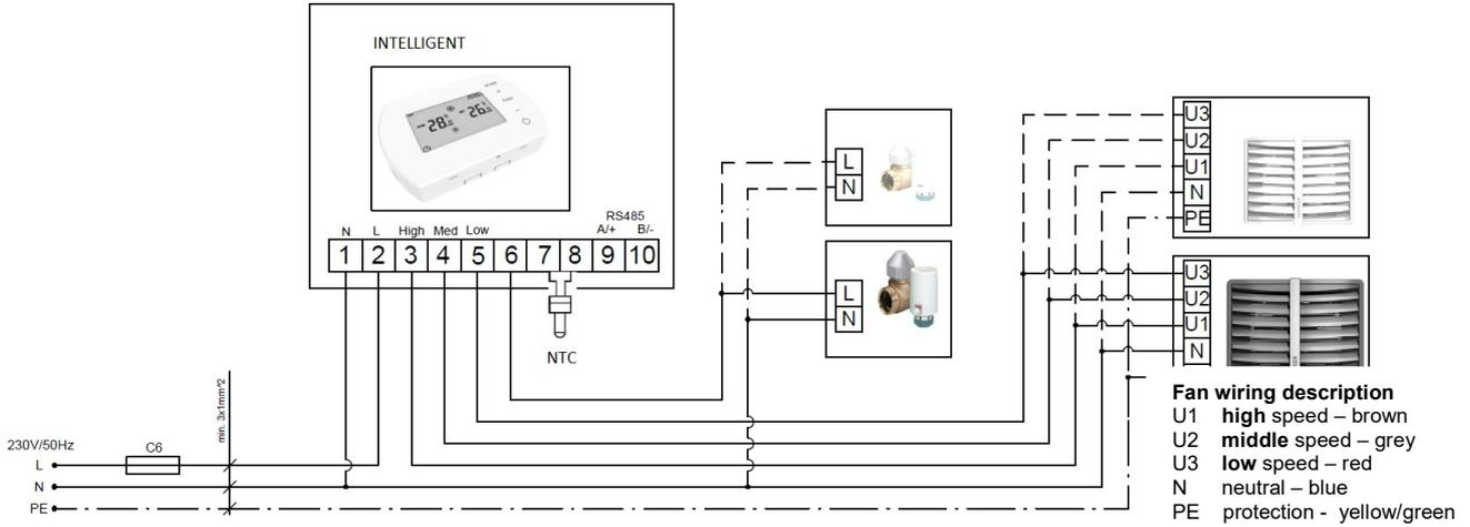
**4. Splitter MULTI 6 - control up to 6 pieces of HEATERS from one COMFORT or INTELLIGENT Panel**
