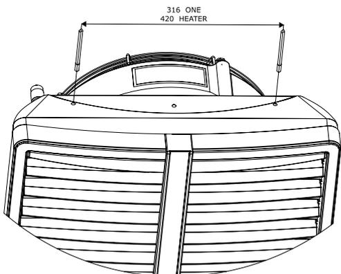
**Installation of mounting pins**
