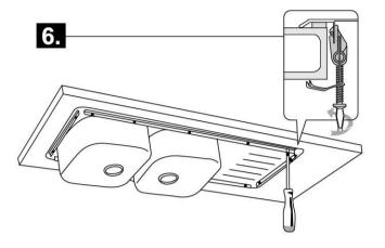
Tighten the screws of the anchor braces (with a hand screwdriver), to secure the sink in place.
