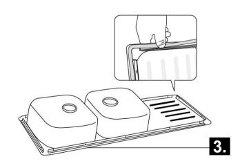
Adhere the seal tape around the under side of the edge of the sink, being careful to lay it smoothly (without ridges).
