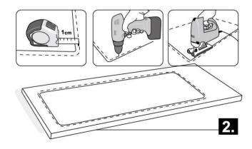
Draw another line 10 mm inside the first line. cut a hole in the counter top following this second, inner, line. (\*if the manufacturer has included a pattern in the package, then use the pattern to cut the hole in the counter top).
