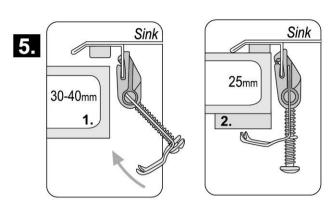
These anchor bracesaredesigned for use with counter tops 30-40 mm thick (1). If your counter top is thinner, insert wooden wedges between the counter top and the braces so as to secure them (2). After placing two at each corner of the sink, place the rest evenly spaced around the perimeter of the sink.
