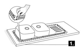
Place the sink upside down in the position where it is to be installed, and trace the outline of the sink on the counter top with a pencil.
