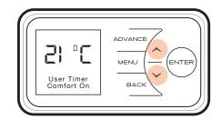
If you require a different room temperature use the **Up and Down** buttons until the display shows the temperature you require.
