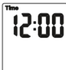
Press Time to set the hour, and then the time will show the minutes. The hour is a 24 hour clock.
