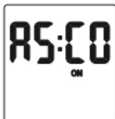
Use the Adv/Ovr button to change between on and off for the automatic summer time adjustment and proceed to section 6.
