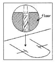
Drill Dia 10mm, min . drill hole depth 60mm
