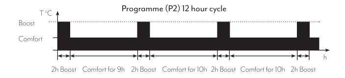
N.B. The maximal temperature during the "Boost" period in "P1" and "P2" mode is limited to 65°C
