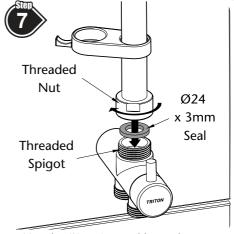
Position the Ø24 x 3mm rubber seal on top of the threaded **Diverter Valve** spigot.
