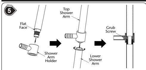
Assemble the **Top Shower Arm** into the **Shower Arm Holder**, note that the **Top Shower Arm** can only be assembled one way, so ensure that the flat faces of **Top Shower Arm** and **Shower Arm Holder** are aligned.
