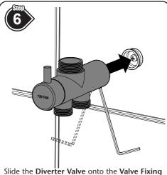
Slide the **Diverter Valve** onto the **Valve Fixing Bracket** and tighten the 2 x **Grub Screws** on the underside of the **Diverter Valve**.
