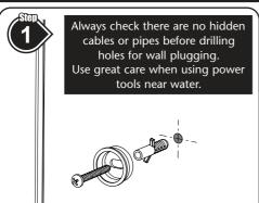
Referring to *Positioning the Dual Outlet Diverter* guidance, mark the wall fixing position for the **Diverter Fixing Bracket** and drill and plug the wall. Ideally the hole should be positioned in the centre of a tile and not in the grouting.
