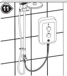
Take the **Short Hose** and fit a hose seal into the conical nut and connect to the **Shower Unit**, fit a hose seal into the conical nut at the other end of the hose and connect to the inlet of the **Diverter Valve**.
