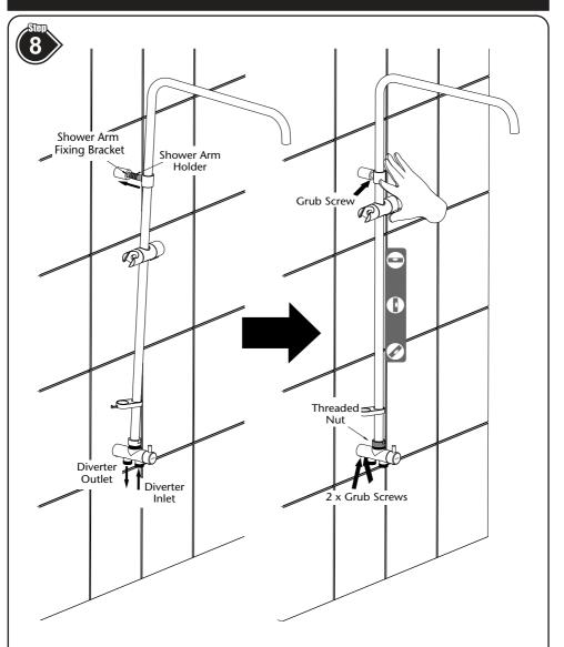
Pivoting the **Shower Arm** slightly away from the wall, slide the stem of the **Shower Arm Holder** into the **Shower Arm Fixing Bracket**.
