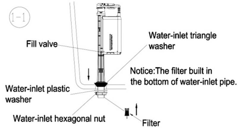
Put fill valve & water-inlet triangle washer insert into water-inlet hole of water tank, then, cover water-inlet plastic washer and hexagonal nut in tum from the bottom of fill valve. Fastening water-inlet hexagonal nut and make a proper adjust according to the size of water tank.
