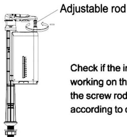
Check if the inlet valve arte working on the rails and adjust the screw rod clockwise according to demands.
