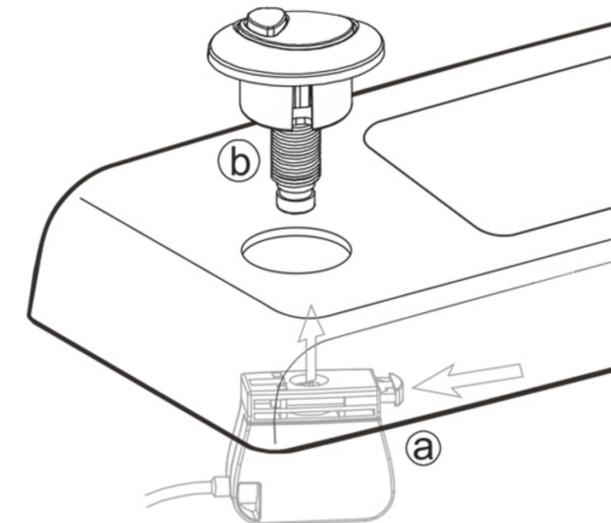
3. Push in the spring lock (a) which is on the control box and then insert button (b) into the control box.
