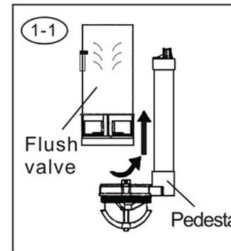
Contrarotate drainage body and make it remove from pedestal.
