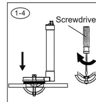
Circumrotate bolt by screwdriver and be sure that seal between sealing washer and the surrounding for outfall.
