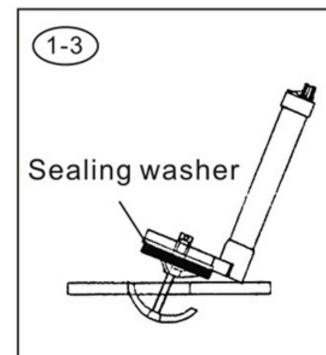
Let pedestal aim at the water tank scupper, deflect properly, circumrotate, and, the stainless steel hook can reach the scupper downside, then, revise the pedestal, the sealing washer should put upside. Go through the pedestal by the middle finger of left hand to keep off stainless steel hook and make its both sides put around the outfall symmetrically.
