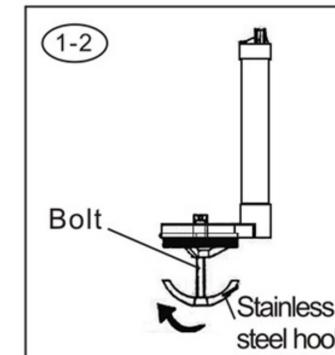
Circumrotate stainless steel hook to the end of bolt clockwise.
