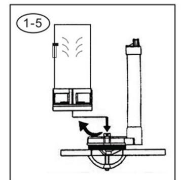
Let flush valve body insert into pedestal and circumrotate it inside the buckle clockwise.
