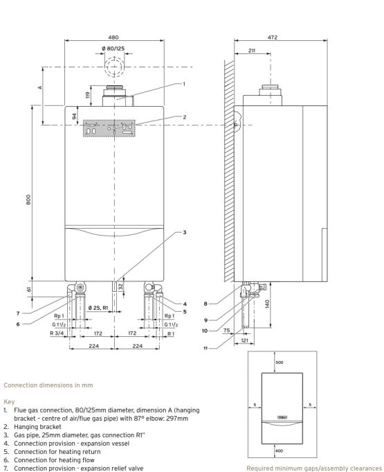
For the installation/assembly of the boiler as well as for carrying out future maintenance tasks, you need the minimum gaps and assembly clearances given above.
