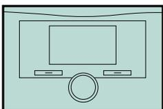
Programmable thermostats are room thermostats that monitor the temperature. As well as having timer programs, they have lower and higher temperature parameters to ensure the temperature doesn't reach an uncomfortable level. This type of control usually also has a holiday function.
