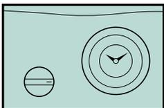
Mechanical timers offer an easy to use, basic solution. Users simply set gears on a dial that turns the boiler on and off at the same time each day.
