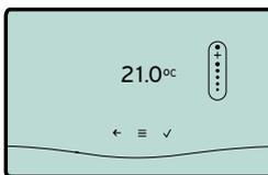
Internet connected controls are controlled remotely and offer the same functionality as programmable room thermostats. These controls have complimentary apps\* so they can be controlled via mobile devices and connect to smart devices, e.g. Amazon Alexa and Apple HomeKit.
