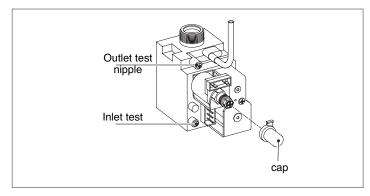
Light the appliance as described in 6.4 INITIAL LIGHTING and compare the reading on the manometer with the values described in 2.2 TECHNICAL DATA. If adjustement is required, follow the detailed instructions in section 8.3 CHECKING AND ADJUSTING BURNER PRESSURE. Once the burner pressure has been checked, isolate the appliance from the electrical supply, remove the manometer, and tighten the gas valve outlet test nipple.
