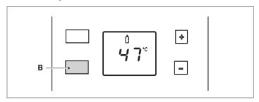
If no action is taken, once 2 minutes have passed the appliance exits the menu and returns to the normal operation screen.
