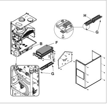
For the conversion from methane gas to LPG, install the burner flange (H).
